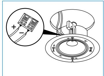
3. Take the speaker unit out of the packaging and remove the grille. Connect the speaker wires to the appropriate "+" and "-" connections (select the desired tappings for 100V units).
