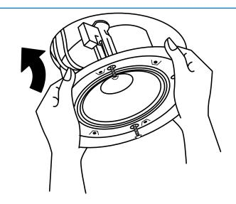
4. Install the speaker unit into the cut-out, ensuring that the 4 dog-ear mounts are turned inwards.
