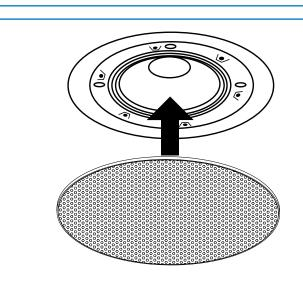
Place the speaker grille back onto the speaker, it will fix magnetically.
