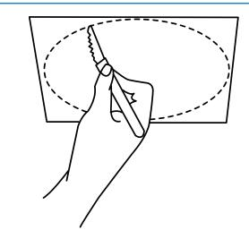
Position the cutting guide against the ceiling where you intend to install the speaker and trace around it.
