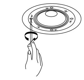
5. Once in place, turn the 4 fixing screws clockwise. This will cause the dog-ear clamps to rotate outwards and tighten to hold the unit in place.
