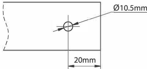
**Note:** When drilling new holes always ensure they are diametrically opposite each other so that the bolt can pass straight through.
