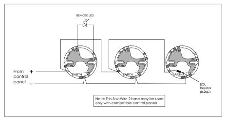
Sav-Wire base wiring diagram
