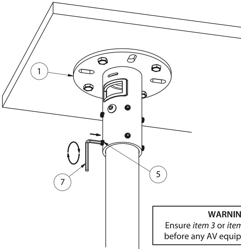
The angle of the pole can be micro-adjusted by adjusting *item 5* with *item 7*.
