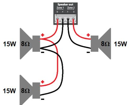
Ensure that the combined impedance connected to each speaker output is not lower than 4Ω and that the speakers connected can handle the output power at that combined load impedance.
