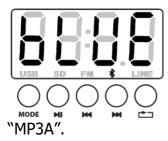
Pressing the mode button until the display shows "bLUE" enters Bluetooth receiver mode.
