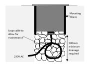
• There must be enough cable below the luminaire to carry out maintenance work (see Fig. 3)
