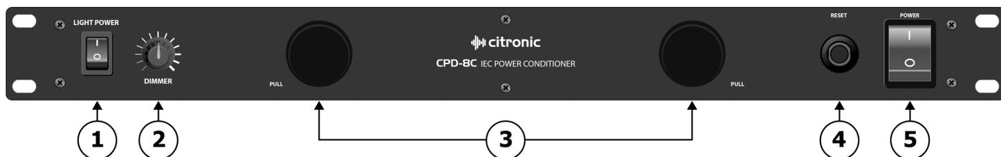
1. On/Off power switch for rack lamps
