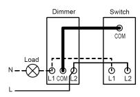
Two-way switching with a dimmer can only be achieved when there is only one dimmer in the system. Two-way dimming cannot be achieved
