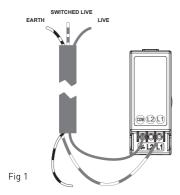
For a multiple gang dimmer repeat the wiring method for each dimmer unit
