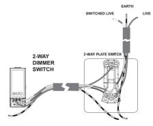
Two-way switching with a dimmer can only be achieved when there is only one dimmer in the system. Two-way dimming cannot be achieved
