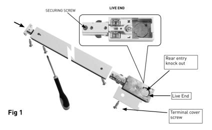
Remove the terminal cover screw from the Live End to gain access to the mains connections
